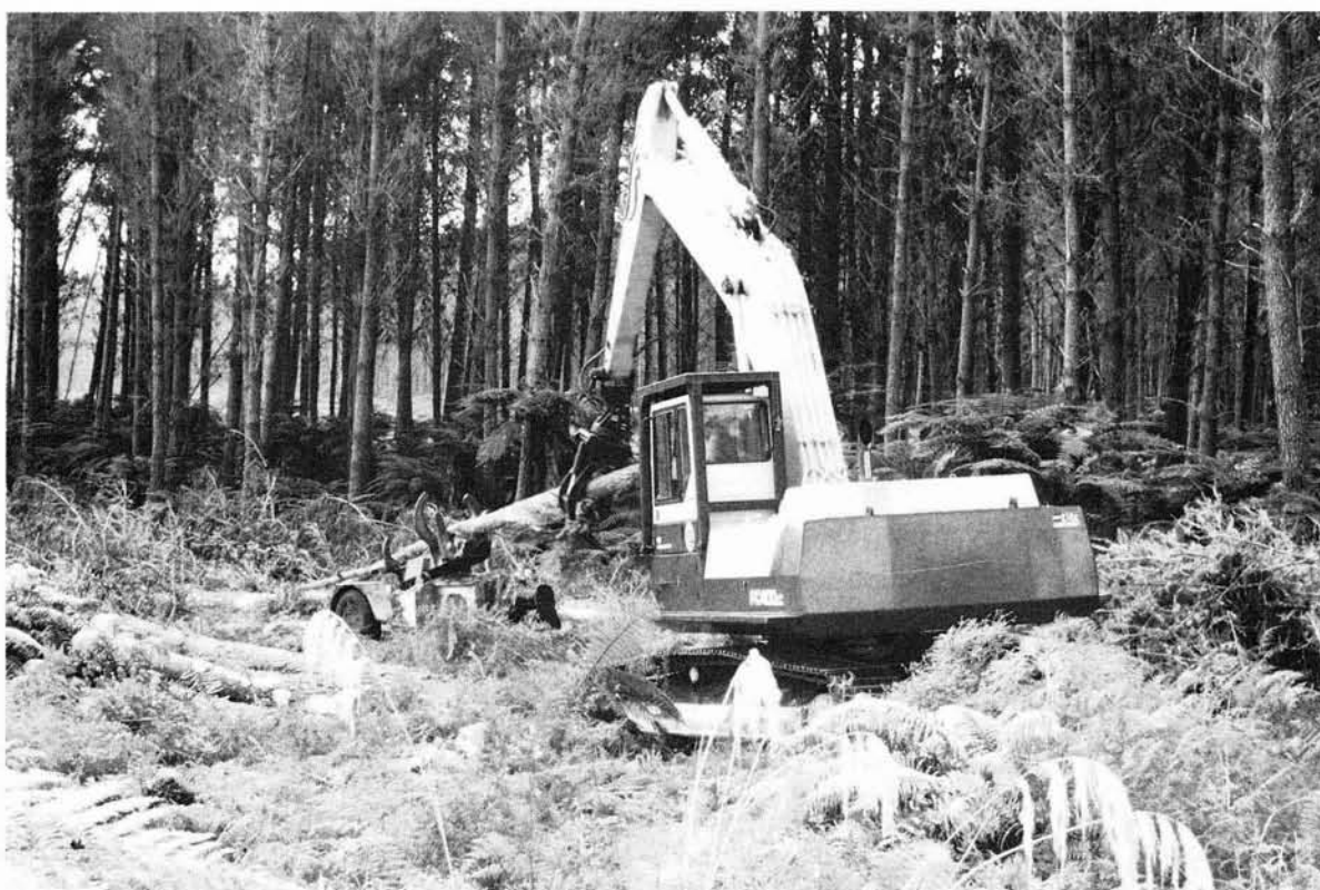
Figure 1 - Komatsu PC400 Excavator and Holmes static delimer in operation
