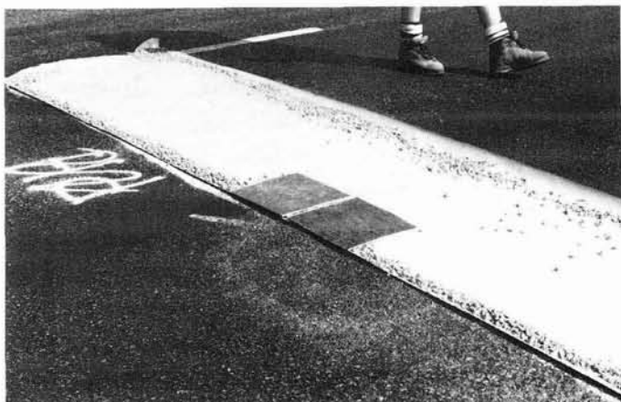
Figure 4 - Carpet mats used to measure bitumen application rate
