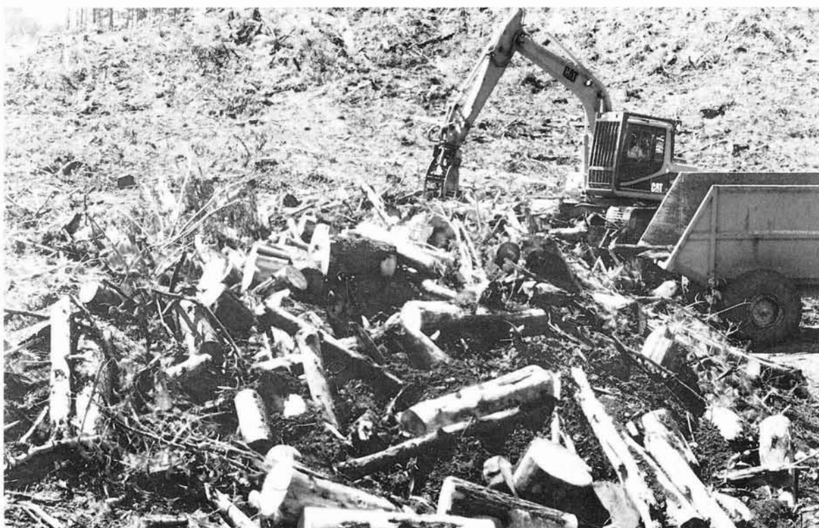
Figure 1 - Cat 311 excavator sorting and stacking waste wood from a skid surround
