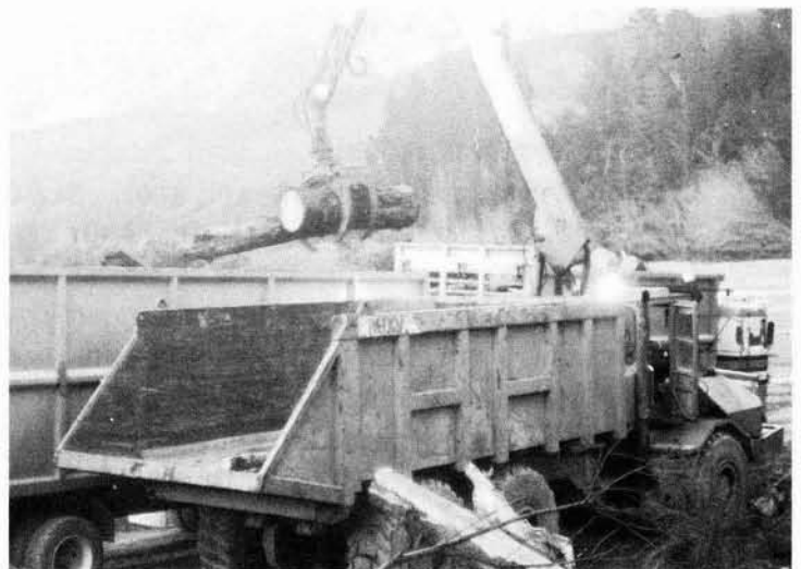
Figure 2 - Bin truck being loaded with waste wood by Moxy off-highway truck fitted with a crane
