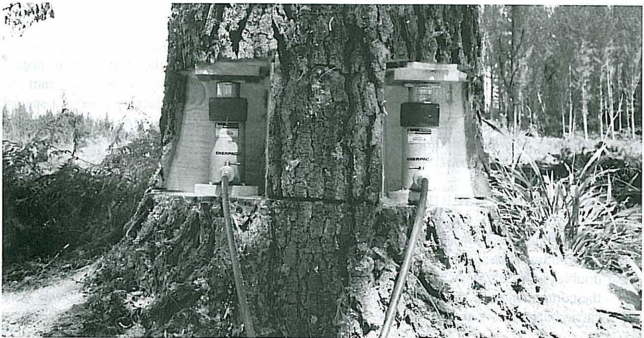
*Figure 1 - Jack cylinders inserted in the back of a tree*
