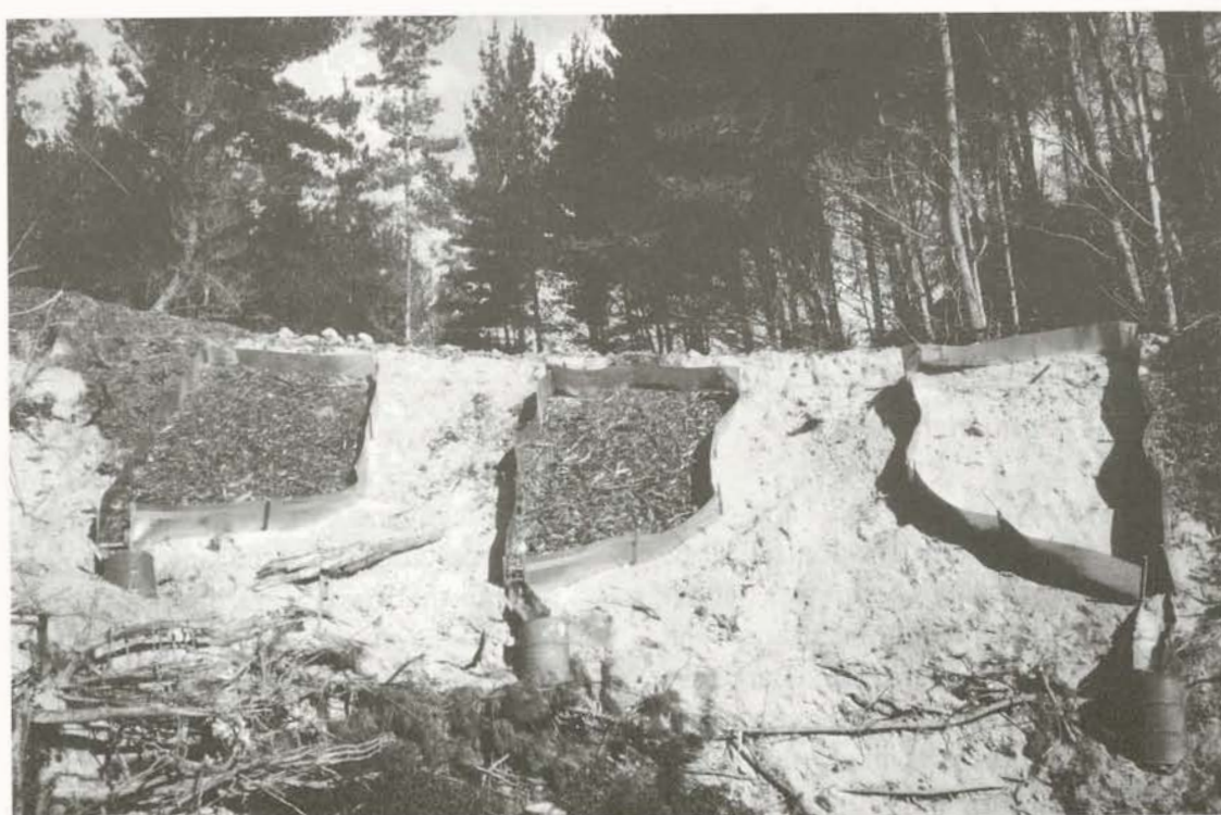
Figure 1- Runoff plots installed on a newly constructed fill slope
