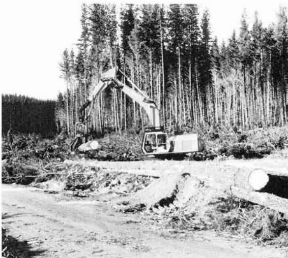
Figure 2 - Waratah 234 tree length delimbing in Tarawera Forest
