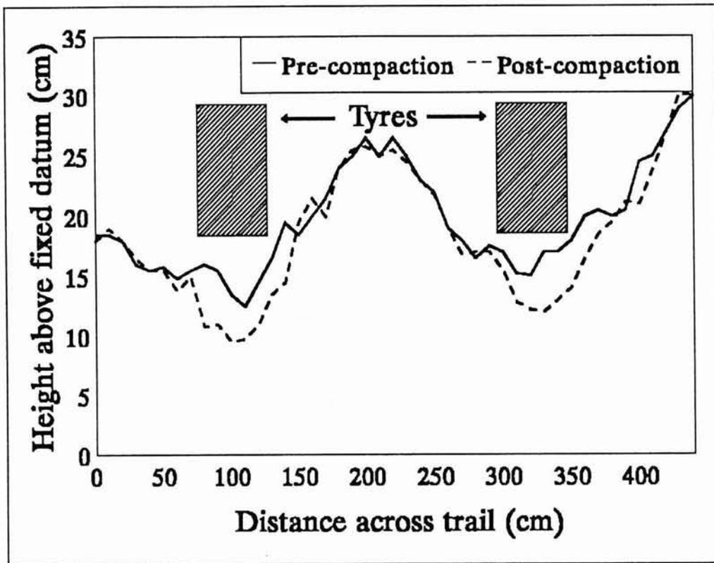
Figure 3 - A surface relief profile showing planting mounds and area of compaction
