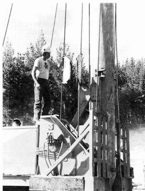
Figure 1 - Remote tension monitor load cells mounted on Bellis hauler
