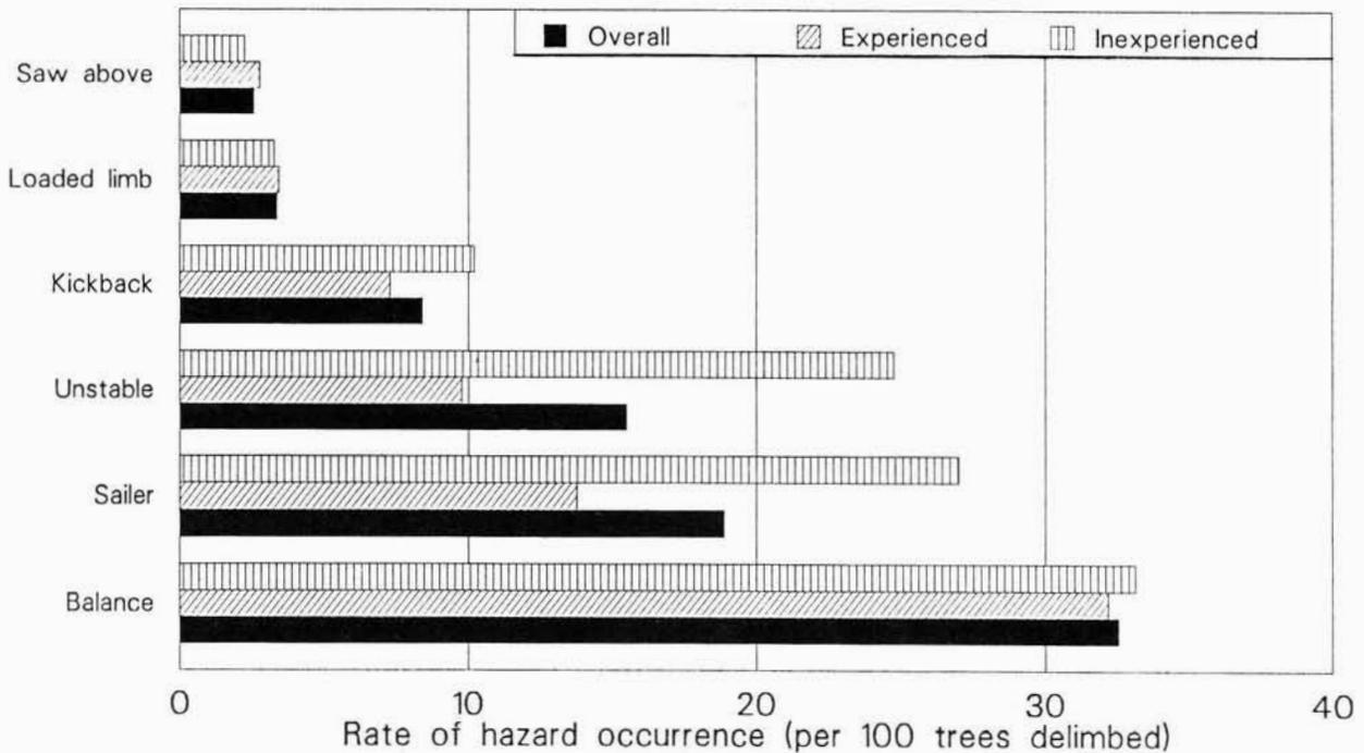
Figure 4 - Rate of occurrence of delimiting hazards (per 100 trees delimited) for inexperienced and experienced loggers
