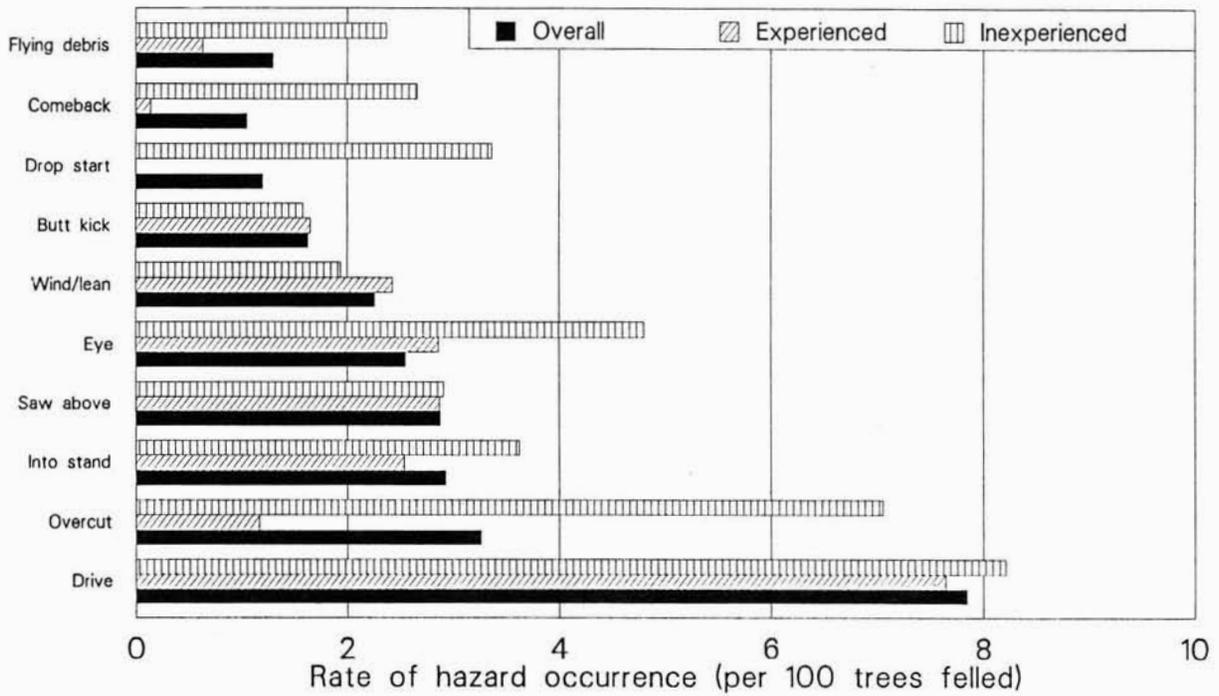
Figure 3 - Rate of occurrence of felling hazards (per 100 trees felled) for inexperienced and experienced loggers
