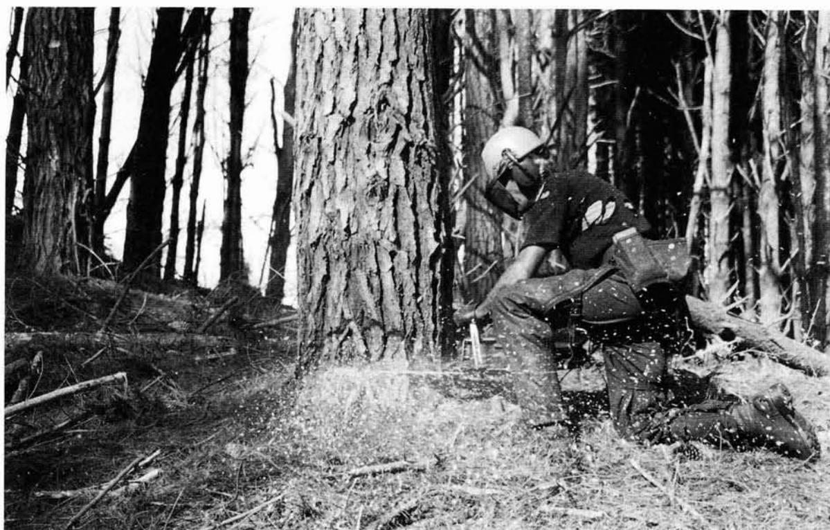
Figure 1 - Faller using his visor to prevent eye injury from the hazard of flying debris
