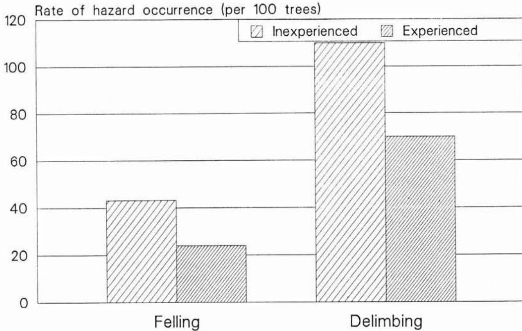
Figure 2 - Comparison of total number of hazards (per 100 trees) confronted by loggers during felling and delimiting
