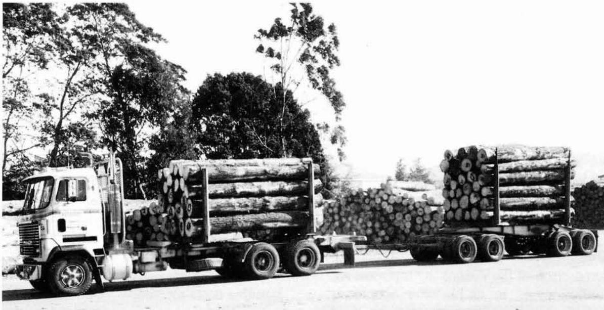
*Figure 1 - 6x4 + 4 axle convertible; now able to load to 44 tonnes under the new regulations*
