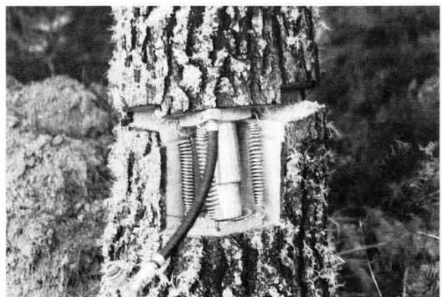
Figure 4 - Cutting technique using a single Silvey ram unit on a small tree with a heavy lean
