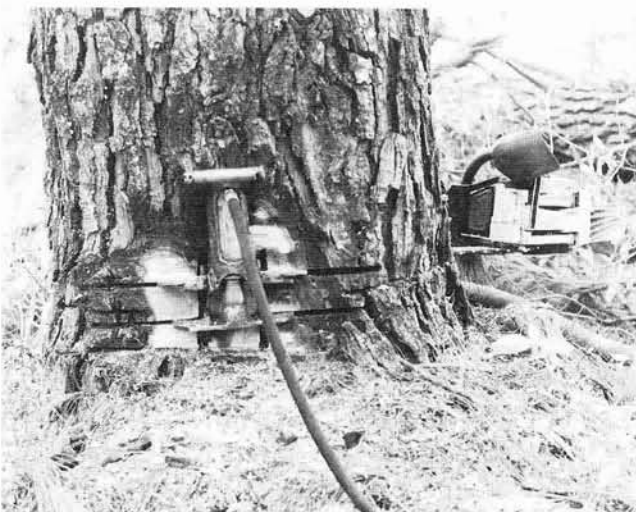
Figure 2 - The Kajavala tree jack and the two vertical and horizontal backcuts
