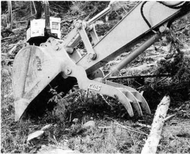
Figure 5 - Excavator boom/bucket with a hydraulic "thumb" for grappling logs
