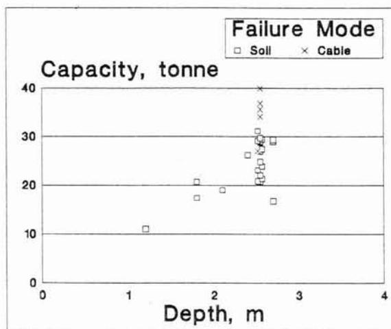
Figure 9 - Capacities for cylindrical anchors tested in California
