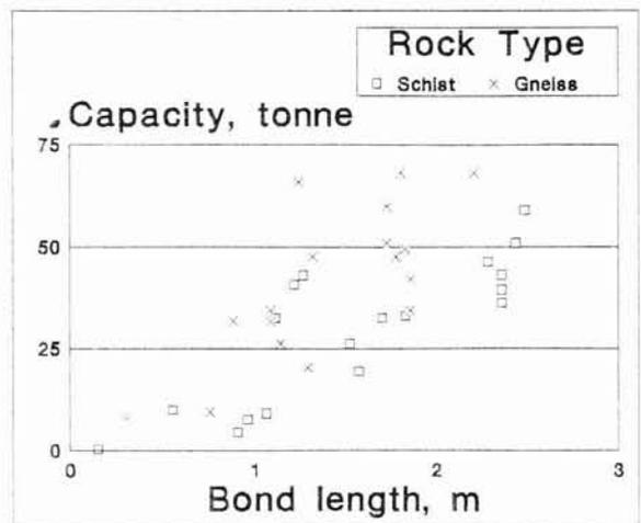
Figure 4 - Pullout capacities for grouted rock anchors tested in Alaska
