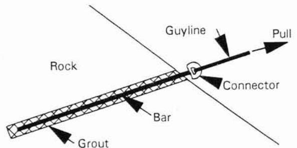
Figure 3 - Schematic of grouted rock anchor and attachment to line
