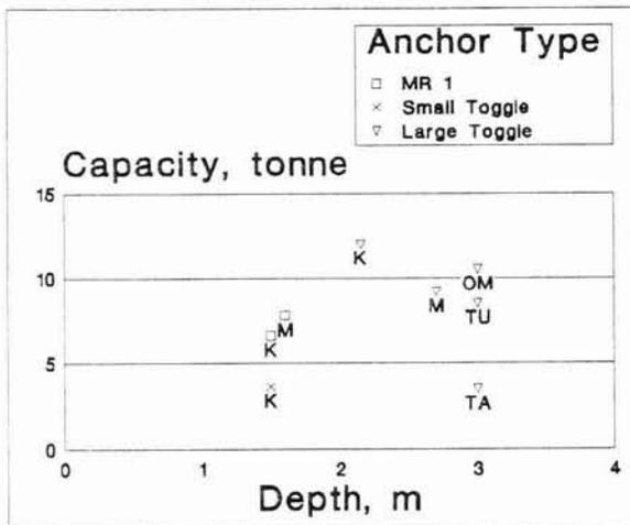
Figure 2 - Pullout results for anchors tested - Kinleith pumice soil (K), Mangatu wet silt (M), Omataroa pumice (OM), Tairua wet clay (TA), and Tuatapere clay with iron pan (TU)
