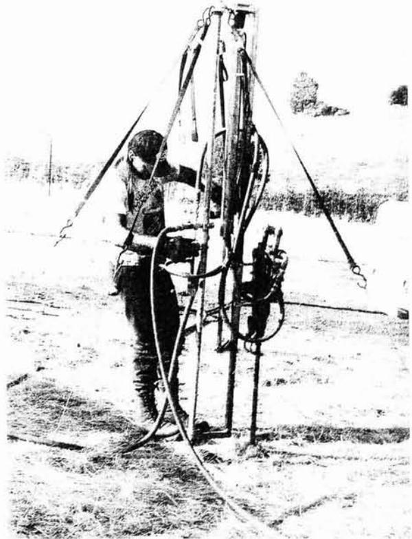
*Figure 6 - 35kg drill and frame*
