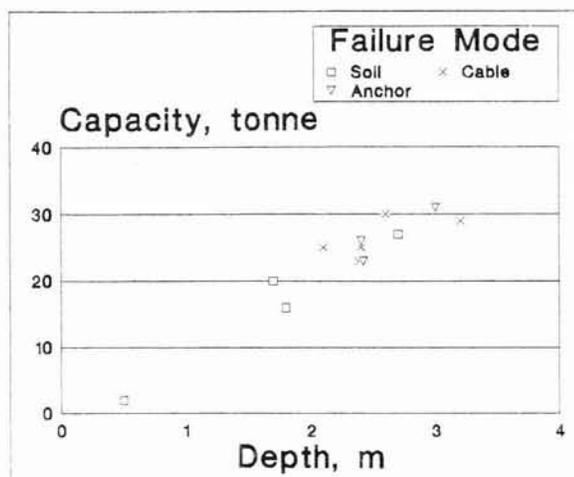
Figure 8 - Capacities for MR2 anchors tested in California and Oregon
