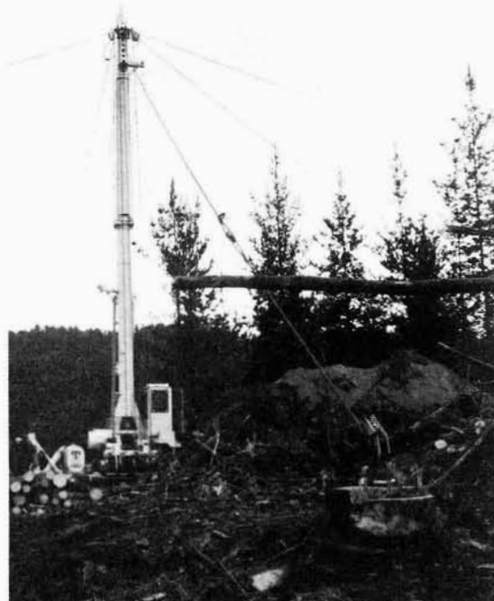
Figure 1 - Madill 171 fitted with LIRO tension monitoring system
