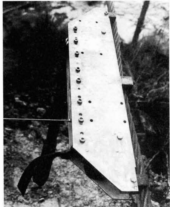
Figure 2 - LIRO dynamometer fitted to the guyline of a Dispatch hauler
