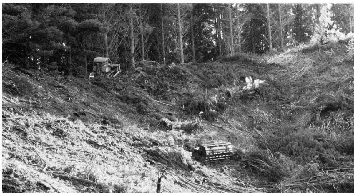
Figure 1 - Gravity roller crushing operation in Omataroa Forest
