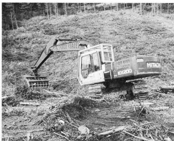
Figure 2 - Excavator with rake clearing dense slash
