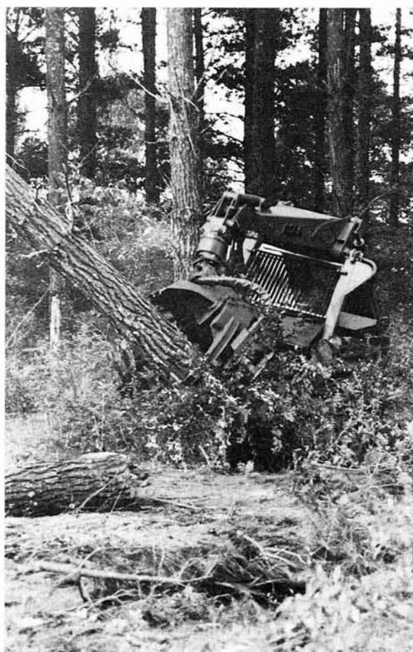
*Figure 1 - Bell Feller-Buncher felling radiata pine*
