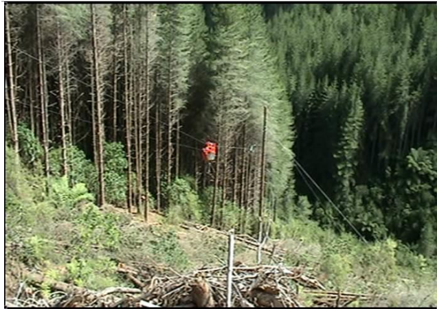
Figure 10. Intermediate support tree (No.2) rigging detail.
