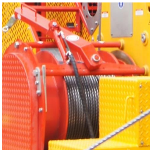
Figure 4: Skyline drum showing narrow tension section and spooling device.
