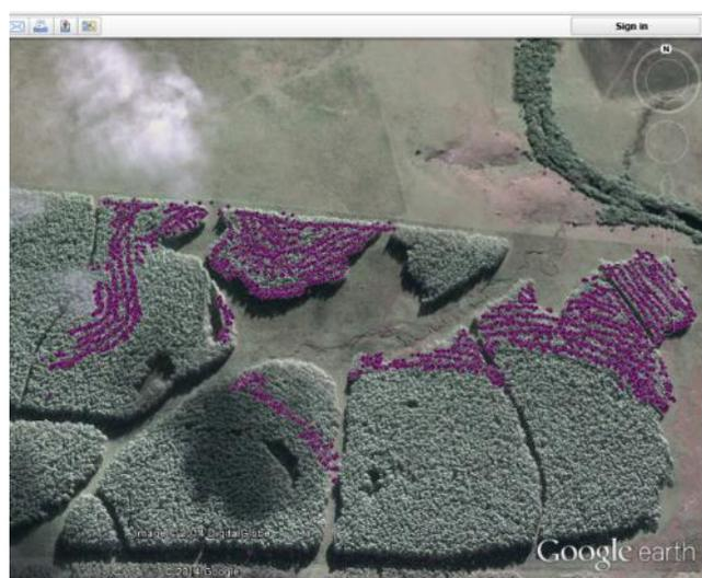
**Figure 3: Visual indication of harvester progress through the stand (each purple dot represents a harvested tree).**
