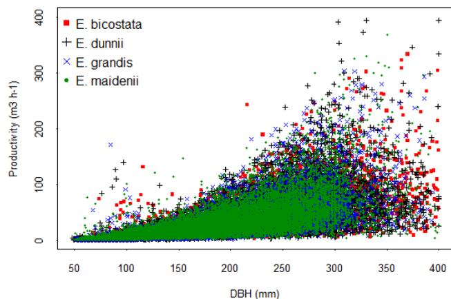
**Figure 5: Graph of productivity per processing hour (all records) as a function of DBH showing distribution of points.**
