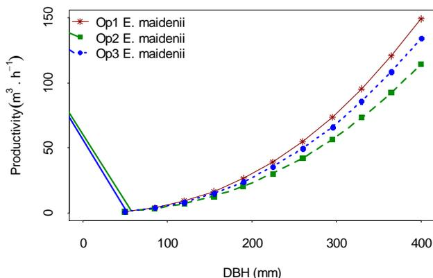
**Figure 7: Operator's productivity predictions by the model for *E. maidenii*. Results expressed per processing hour.**
