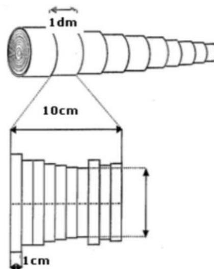
**Figure 4: Stem files record diameter at 10-cm intervals for the whole stem, as well as number and grade of logs cut from each stem.**
