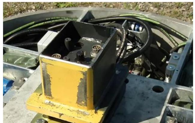
**Figure 2: Fiberdrive attachment showing hydraulic couplers**
