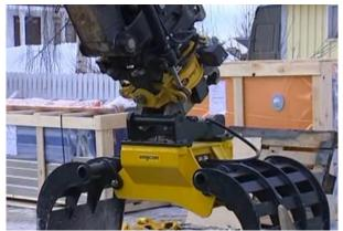
Figure 5: Engcon Automatic hydraulic quick coupler
