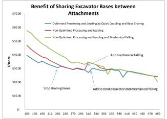
Figure 3: Logging cost (\$/t) over varying production rates for Scenario 1 (red), Scenario 2 (blue) and Scenario 3 (green). Scenario 1 (the red line in Figure 3) shows the operation with no base sharing where new equipment is taken on when required. As new equipment is added there is a spike in cost due to it not being fully utilised.
