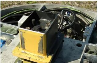
Figure 2: Fiberdrive attachment showing hydraulic couplers
