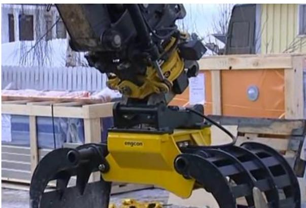
**Figure 5: Engcon Automatic hydraulic quick coupler**
