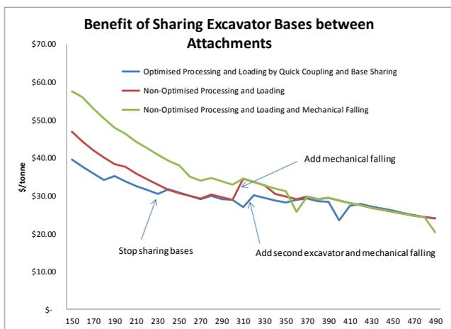
**Figure 3: Logging cost (\$/t) over varying production rates for Scenario 1 (red), Scenario 2 (blue) and Scenario 3 (green).**
