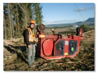
Figure 2: Boman Z7850 motorised carriage with radio controlled drop line.
