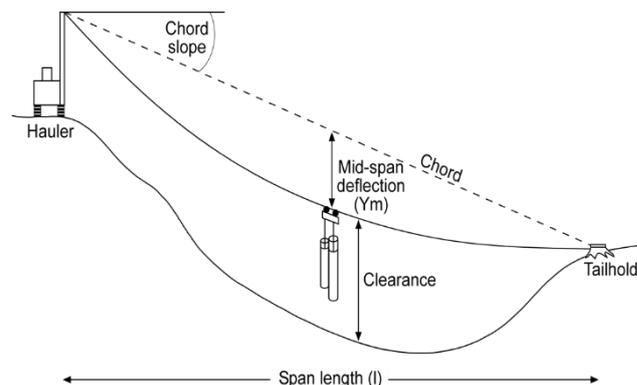
**Figure 1: Measurement of deflection**
