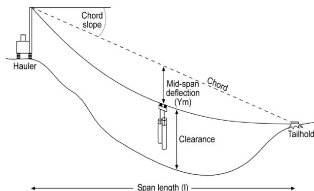
**Figure 1: Measurement of deflection**
