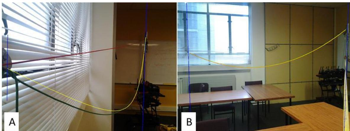
Figure 3: LineSmarts photo processing from Lab Test 1: Photo taken at tail hold (A) and from side (B), showing support positions and estimated shape of skyline catenary.
