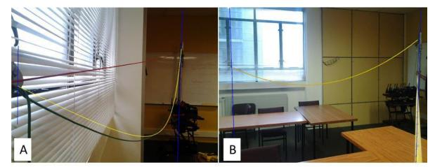
Figure 3: LineSmarts photo processing from Lab Test 1: Photo taken at tail hold (A) and from side (B), showing support positions and estimated shape of skyline catenary.
