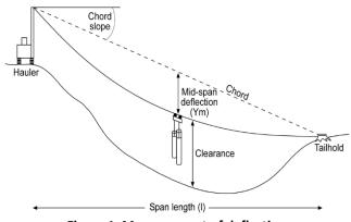
Figure 1: Measurement of deflection
