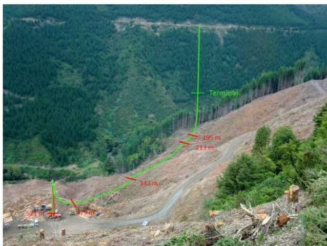
Figure 6: Example of inspection points along skyline span
