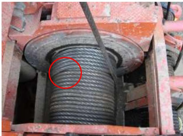
**Figure 8: Example of cross-over points when spooling multiple layers onto drums.**
