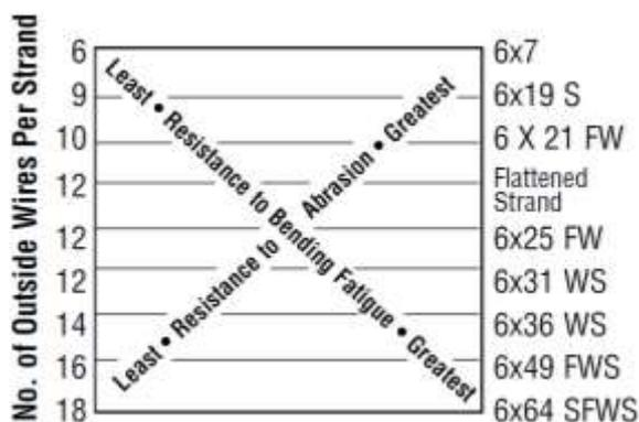
**Figure 1: The "X-Chart" demonstrates the inverse relationship between fatigue and abrasion resistance in wire ropes (Hanes Wire Rope Supply).**
