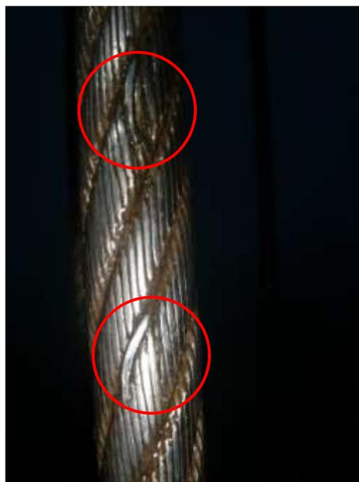
Figure 7: Example of broken wires found during inspection after 6 months of use
