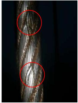
Figure 7: Example of broken wires found during inspection after 6 months of use
