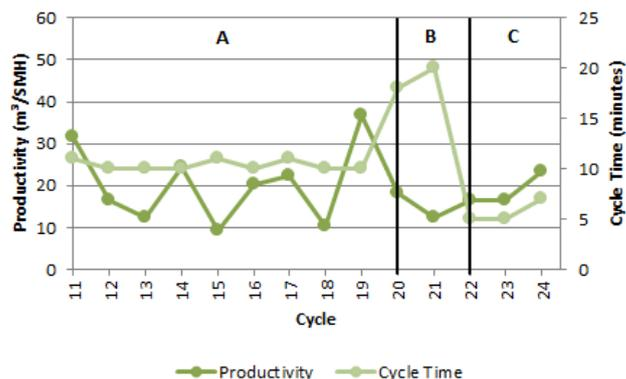
**Figure 6: Production control chart for cycles 11-24 (“Study”) for the crew using North Bend.**
