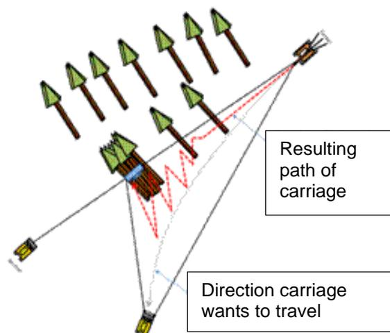
**Figure 10: Effect of bridling on carriage flight path during outhaul.**
