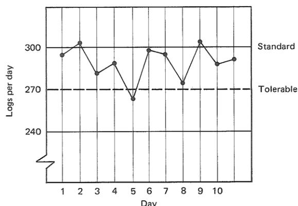
Figure 1: Example of production control chart for cable logging (Conway 1982).
