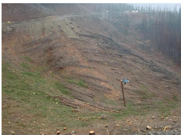
**Figure 7: Side view of span for crew using Falcon carriage. Note the surge pile beyond mid-span.**
