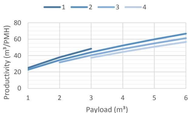
**Figure 9: Relationship between productivity and payload for different number of skyline lifts (at haul distance of 130m and >25% deflection on a 230m span).**
