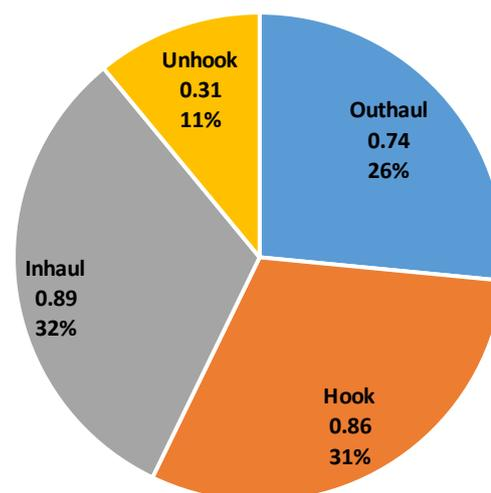
**Figure 8: Observed cycle time components for Falcon Forestry Claw carriage studied.**
