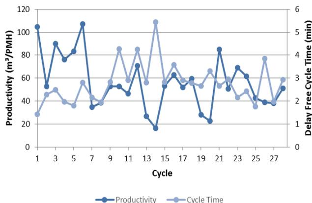
**Figure 11: Production control chart for the study period with the crew using Falcon Slackline.**
