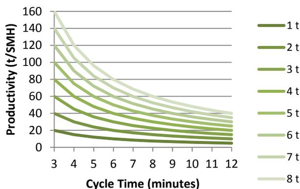
**Figure 2: Productivity and the relationship with cycle time and payload.**
