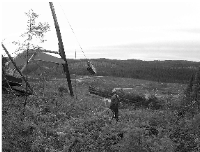
Figure 1. The TLD3000 cable yarder extracting bunches of trees prepared by the feller-buncher.
