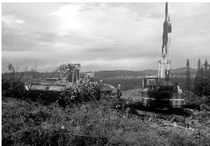
Figure 2. The grapple skidder bringing bunches of trees to the cable yarder.
