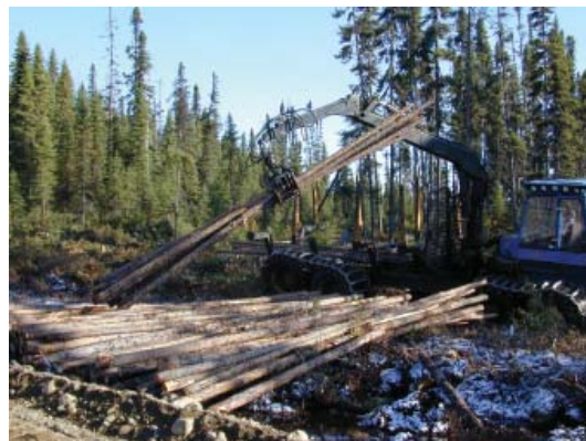
Figure 5. A forwarder loading 7.3-m logs.
