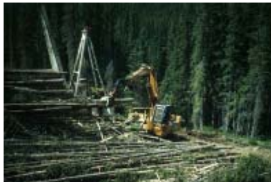
Figure 8. The loader pulling down stems in a high yarder deck for the processor in Block 4.
