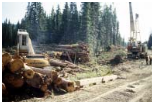
Figure 9. The loader moving the stems to roadside before processing due to a creek in Block 5.
