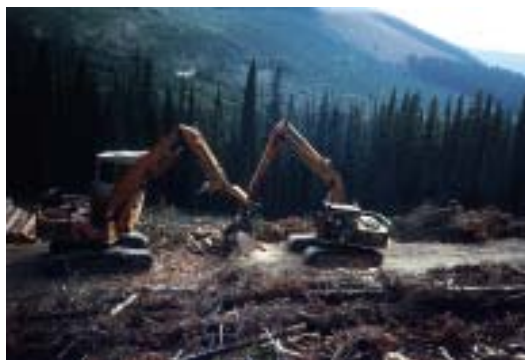
Figure 3. The loader assisting the processor by pulling a large stem into position for processing.
