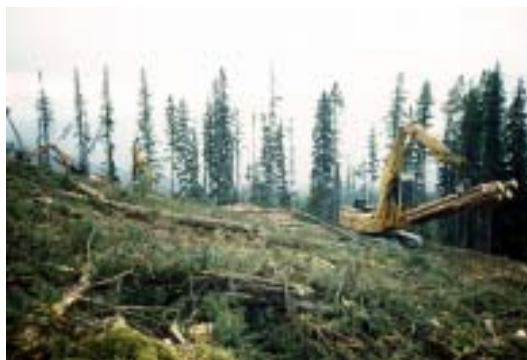
Figure 2. The loader moving processed logs to a suitable decking area.
