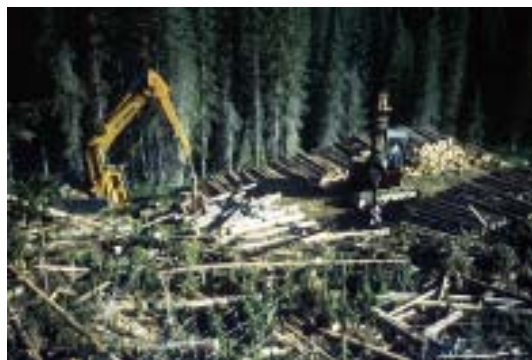
Figure 7. The processor always processed and placed the logs on the left side of the machine due to visibility.
