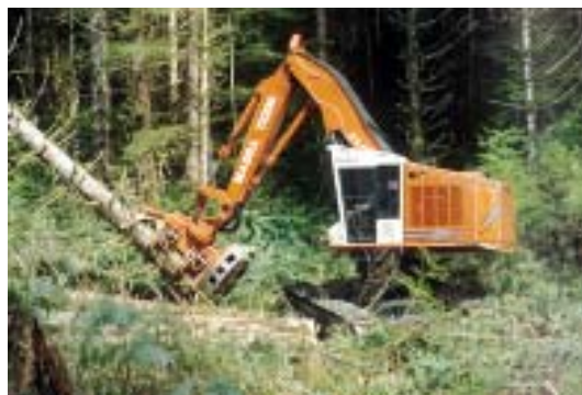
Figure 3. Madill T2200 feller-buncher equipped with a Quadco 2800 intermittent low-speed saw head.
