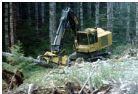
Figure 4. Tigercat 860 feller-buncher equipped with a Quadco 22 high-speed saw head.
