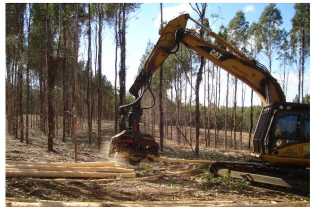
Waratah HTH620 head and operated by an experienced operator. Product specification focused on the production of 5.2m logs to a minimum small-end diameter of 50mm.
