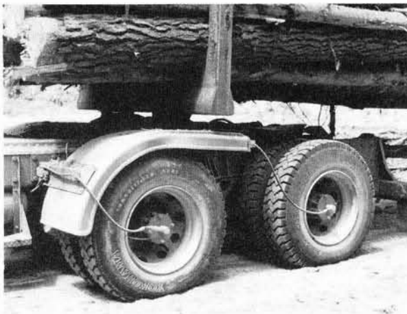
Figure 5 - Air supply hoses and rotary couplings on the drive tyres
