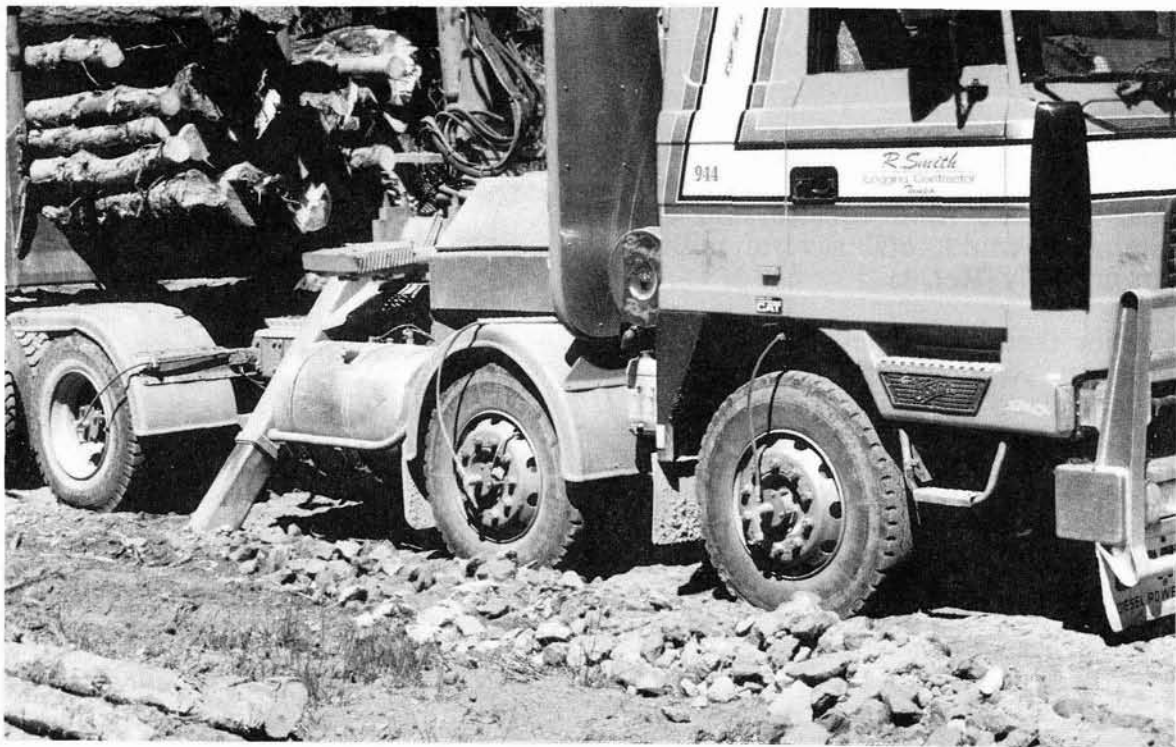
Figure 1 - The New Zealand prototype CTI system fitted on the logging truck
