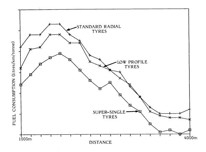
Figure 1 - Comparison of Relative Fuel Efficiency of Tyres (results adjusted for GVW)
