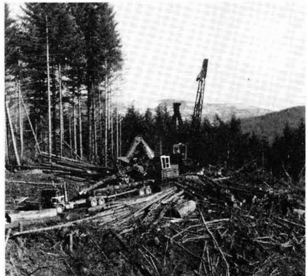
Figure 1 : Efficient landing activities are essential for high productivity with swing yarders.
