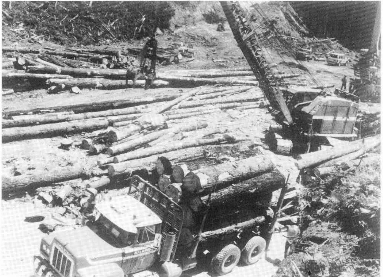
Figure 4 : Rope Crane loading and removing processed logs from the landing chute
