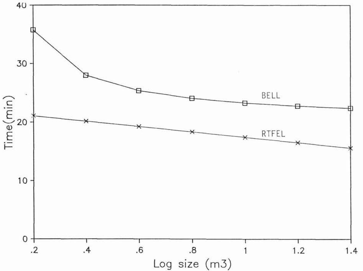
Figure 2 : Predicted Truck Loading Times for Bell Loggers and Rubber-tyred Front-end Loaders for a 30 tonne payload
