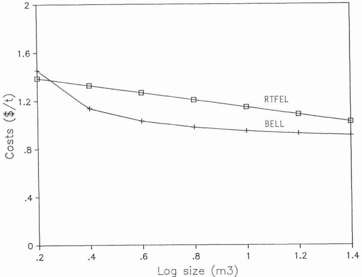
Figure 3 : Comparative Loading Costs for a 30 tonne payload
