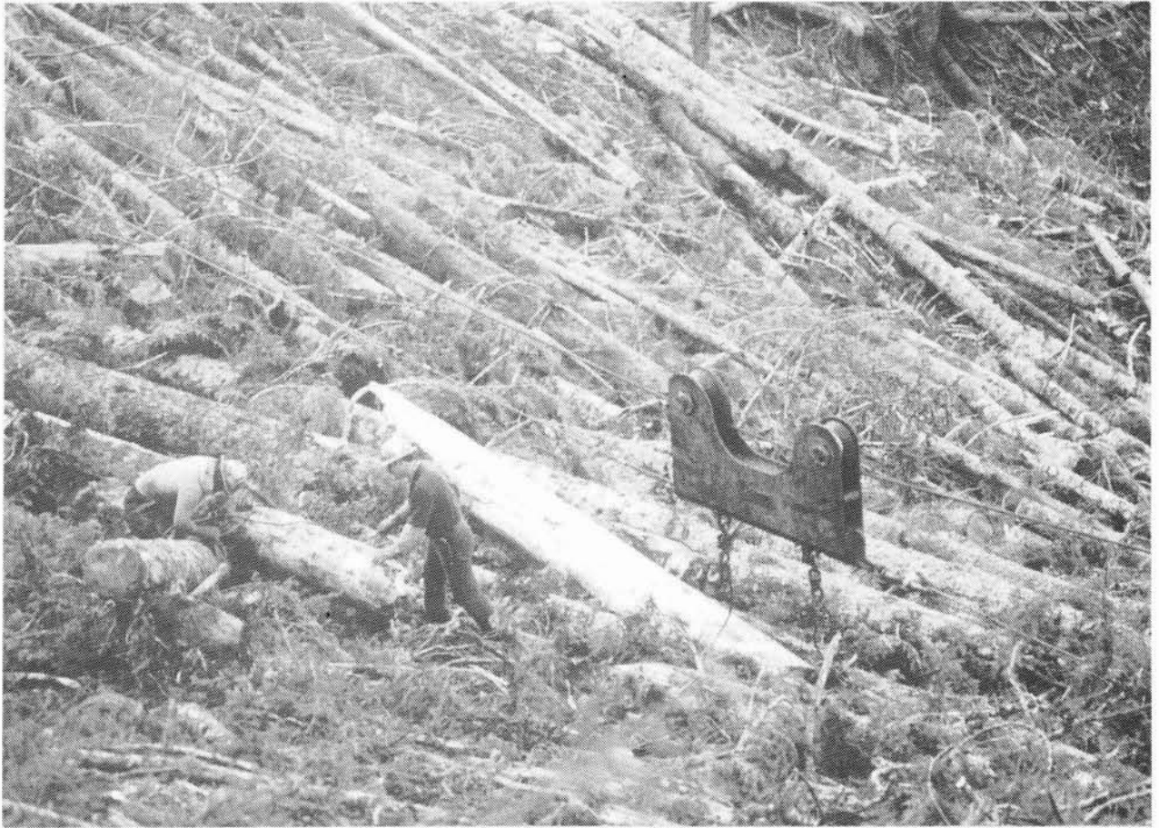
Figure 2 : Two 9 m long strops were used on the carriage with the slackline system.
