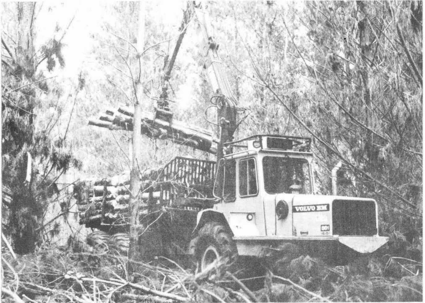
Figure 2 : Volvo 861 Forwarder loading Shortwood
