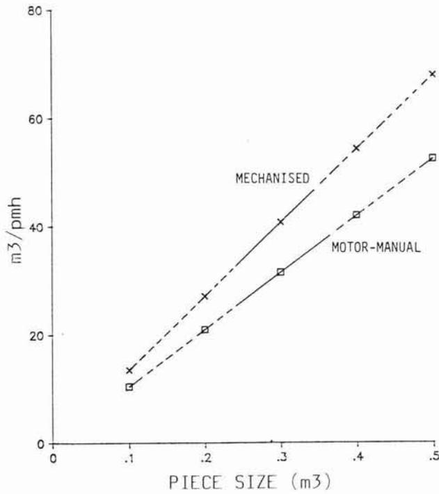
Figure 3(a) : Bunching Productivity System Difference - Same Piece Size
