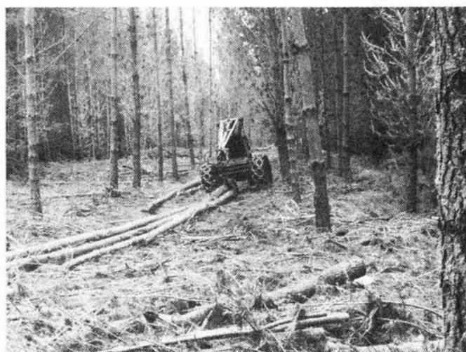
*Figure 1 : Bell Logger bunching logs processed by Lako 3T harvester in an outrow system*
