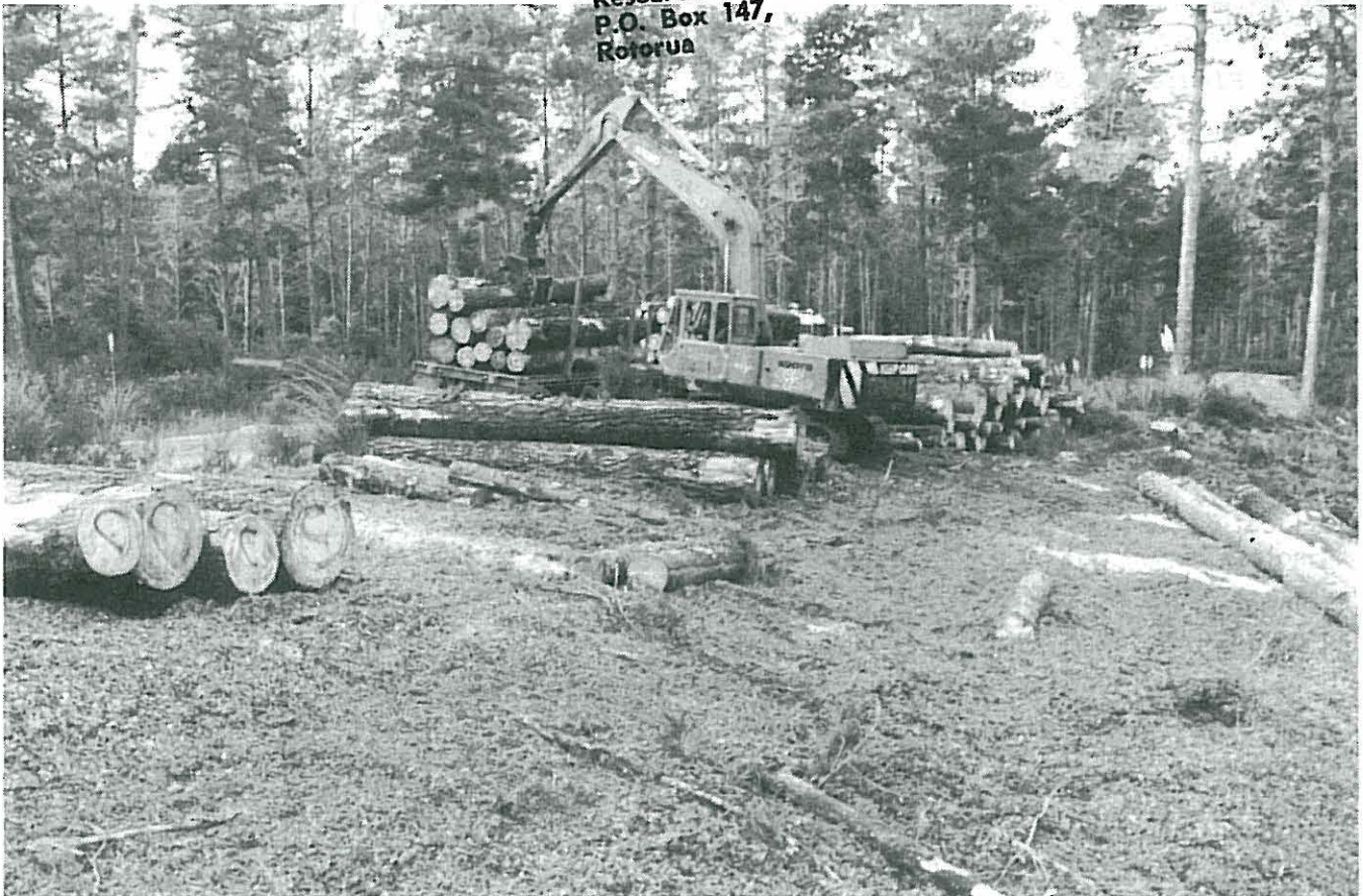
Figure 1 - Hydraulic knuckleboom loader sorting multiple log sorts
