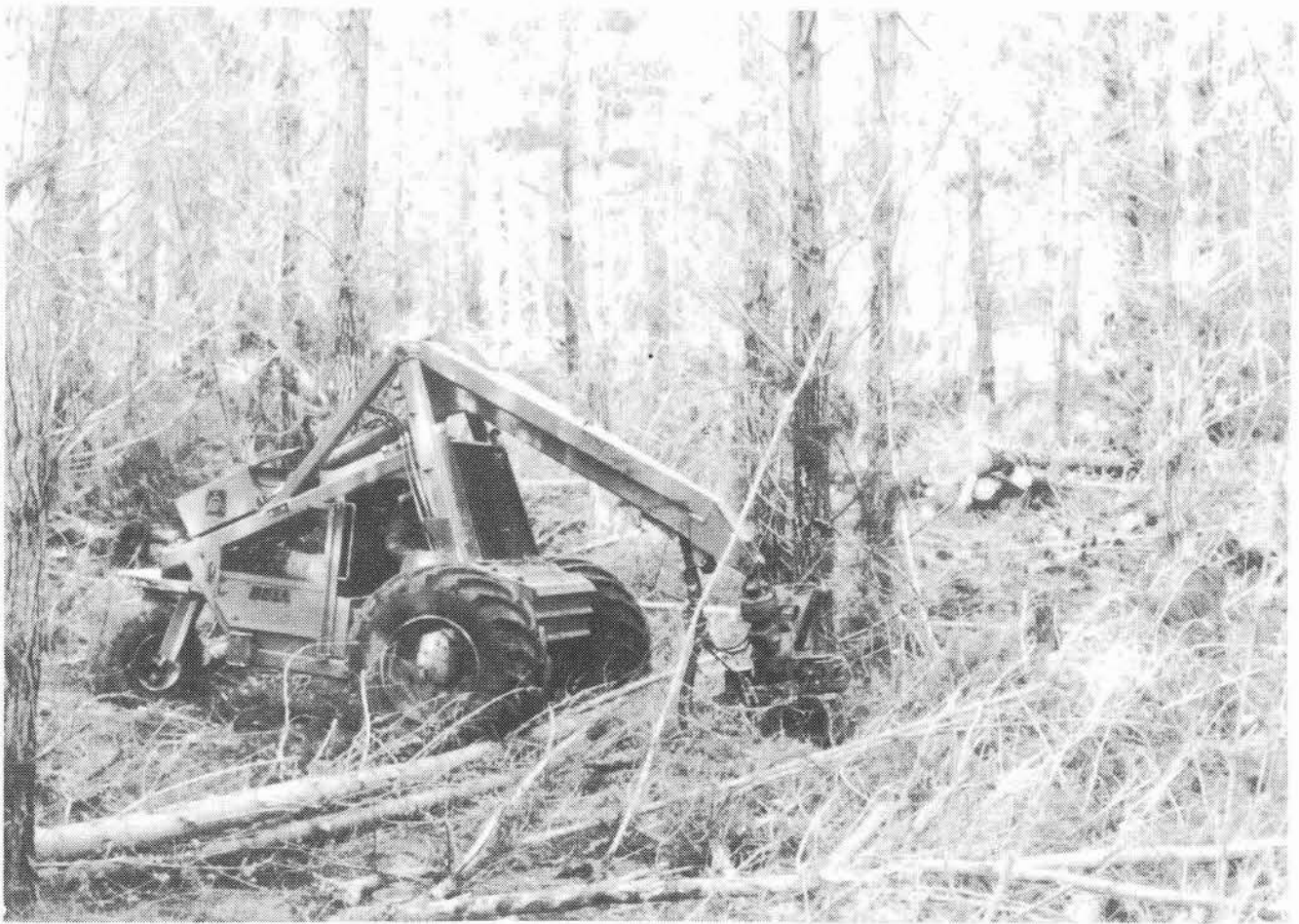
Figure 1 - Bell Logger felling and bunching on Matakana Island
