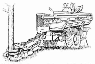
by four wraparound knives and one fixed knife mounted on a winch-driven carriage, which rides along this boom. The carriage incorporates a topping shear and on completion of processing, logs are placed on to an accumulating bunk.
