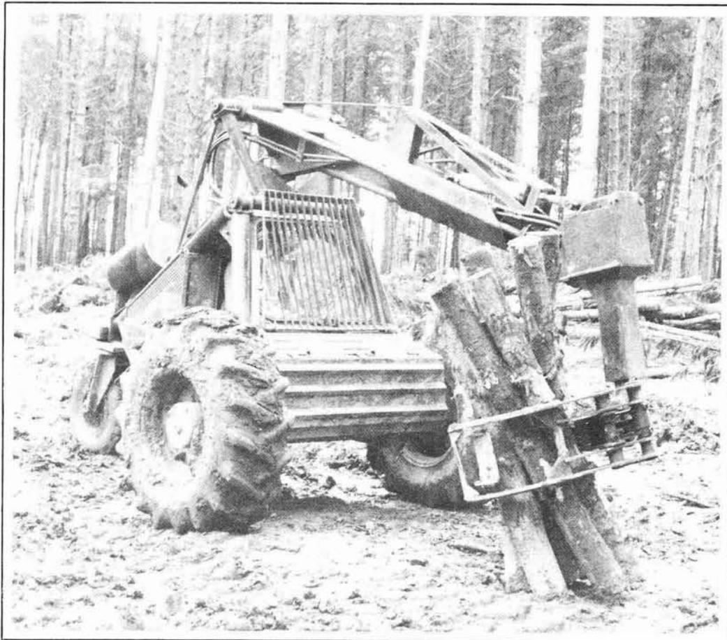
Fig. 1 - Bell Logger fitted with Sunnex boom
