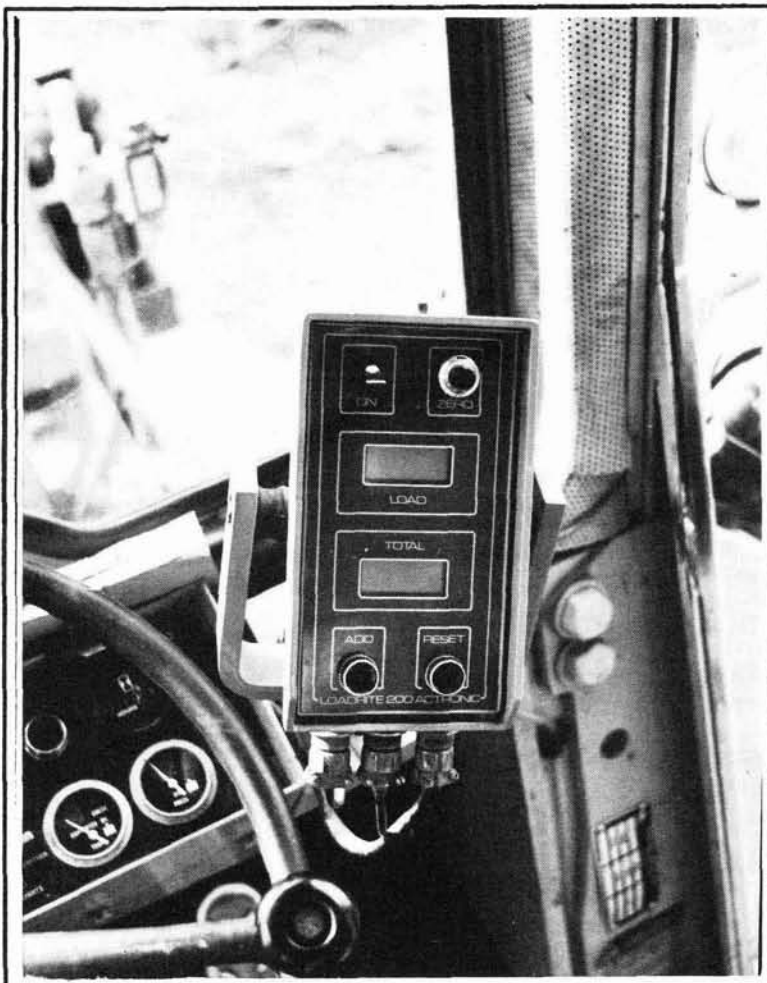
The Loadrite System read-out control box in the cab of a log loader
