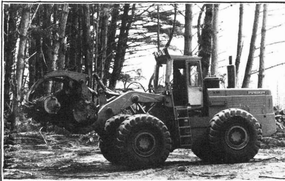
Figure 1 - Loader fitted with the Loadrite system weighing marked logs previously checked by LIRA
