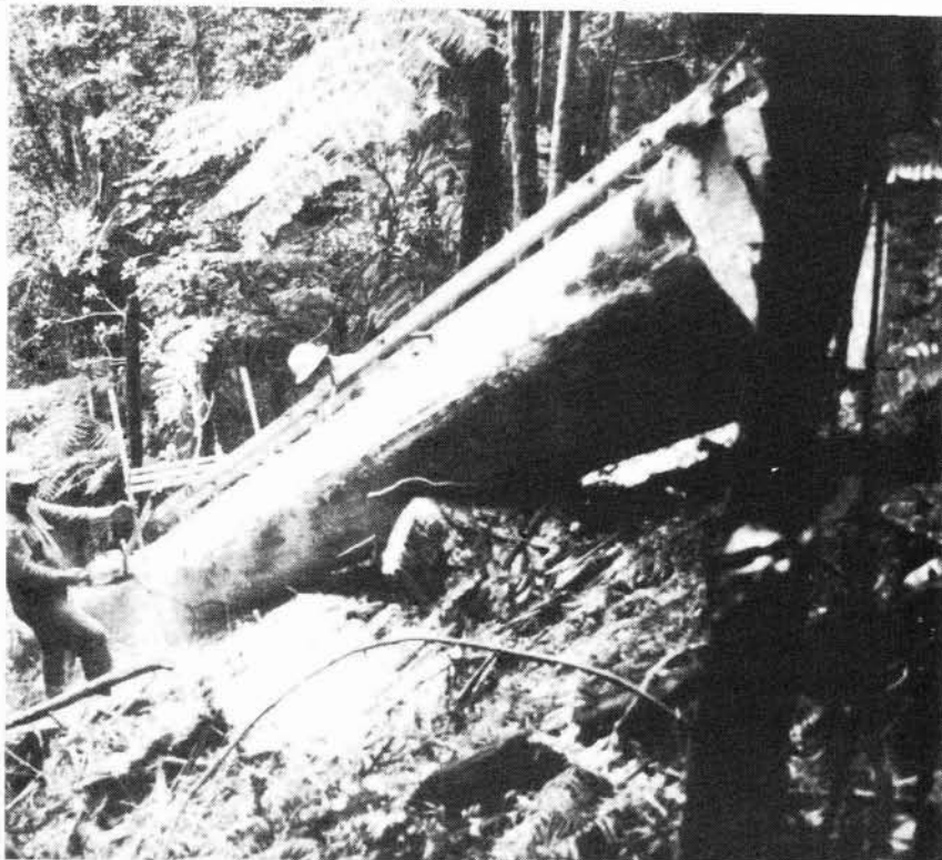
Alaskan mill cut large logs into planks
